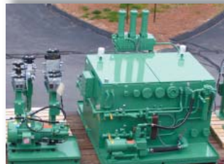
Hydraulic power unit and manifold stands
