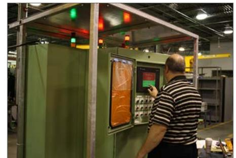
*The electronic control enclosure, which was programmed by The Hope Group engineers, is equipped with a stack-light assembly consisting of green, amber and red indicator lights, with each light indicative of the overall status of the three pump stations.*
