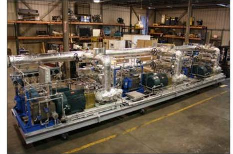
*The compact design of the skid accommodated three pump/motor combinations working in parallel, each pump drawing oil from a common supply and discharge header and each pump/motor has its own electrical controls and protective devices*
