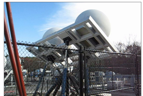
The re-designed and re-manufactured positioning table replicates shipboard pitch, roll and yaw, permitting successful testing of new radar antennas.
