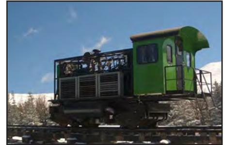
*The fleet of new Cog Railway locomotives are powered by a hydrostatic drive system, all controlled by an electronic joystick.*
