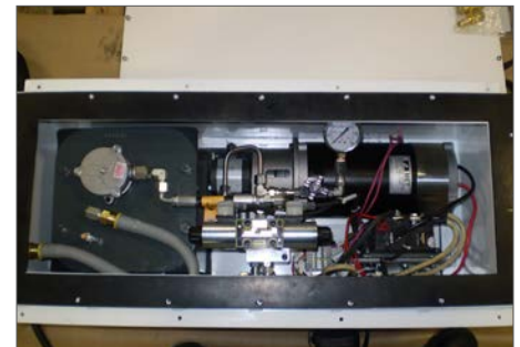
Hydraulic power units were custom designed and built by The Hope Group to provide load leveling to assist in loading vehicles on aircraft.
