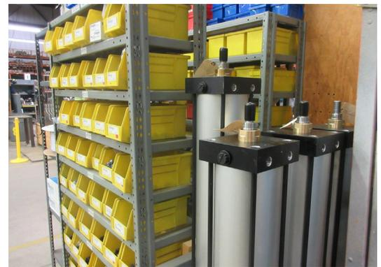
iZap bar code ordering brings the cylinders, fittings, electrical components, and tubing to the Kanban floor at the time of need.
