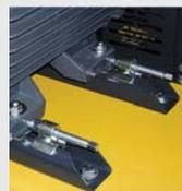
A simple slide based v-belt tensioner makes it easy to adjust belt tension and avoid misalignment.
