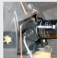
A forced lubrication system provides increased reliability and service life of the pump. Full-flow filtration extends the oil change interval.
